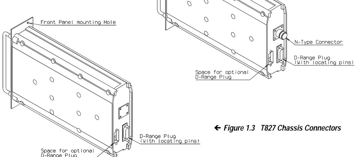
**← Figure 1.3 T827 Chassis Connectors**
